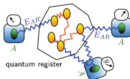
FIG. 1. (Color online) Illustration of an ancilla-driven computation on a register consisting of several qubits. A single ancilla,  $A$ , is sequentially coupled to one, or at most two, register qubits,  $R$  and  $R'$ , etc., and measured. The coupling,  $E_{AR}$ , is fixed throughout the computation while the measurements on the ancilla, indicated by the arrows, can differ.
