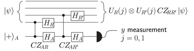
FIG. 3. Ancilla-driven implementation of a controlled-Z gate,  $CZ_{RR'}$ , on two register qubits  $R$  and  $R'$ . Both register qubits are coupled with  $E_{AR(A R')} = H_A H_{R(R')} CZ_{AR(A R')}$  to the ancilla which is then measured in the  $y$  basis. The corrections  $U_R(j)$  and  $U_{R'}(j)$  are local and can be applied through ancilla-driven single-qubit rotations.
