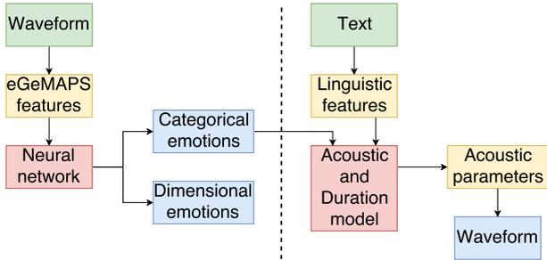
Figure 1: *Controllable SPSS system using external data. In the left half of the figure, an emotion recognition model is trained on external data. In the right half, the predicted labels are used as auxiliary features in a DNN-based speech synthesiser. Green boxes indicate inputs, yellow boxes indicate intermediate data representations, red boxes indicate models, and blue boxes indicate outputs.*
