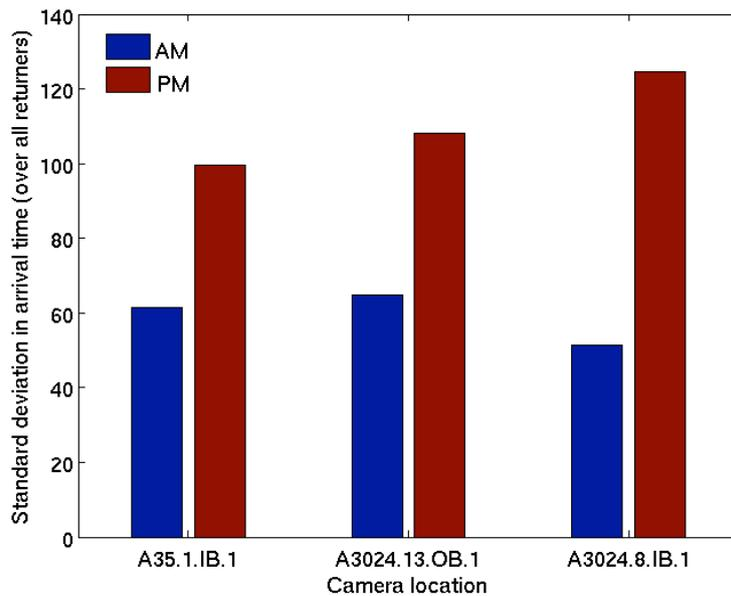
**Figure 5. Standard deviation in arrival times (minutes) at three camera locations in Southampton for vehicles being seen 40 times or more over the 19 week survey period. (A35=9i; A3024.13=4o; A3024.8=2i in Figure 1)**
