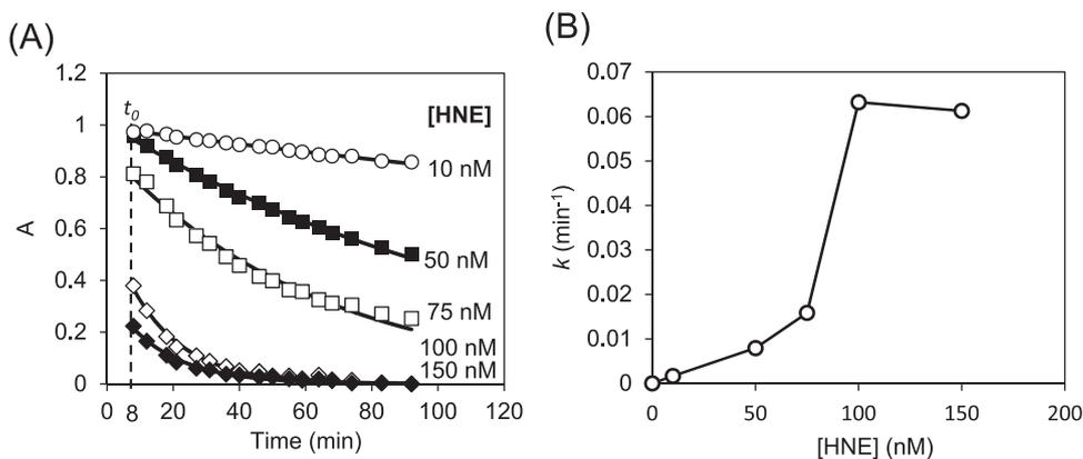
**Fig. 3.** (A) Fractional cleavage vs time plot for substrate-modified electrode cleavage from Fig. 2A upon immersion in different HNE concentrations, being  $t_0 = 8$  min. Solid lines represent the best non-linear fit according to Eq. (2). (B) Variation of the effective constant rate,  $k$ , obtained from fitting the data as a function of the HNE concentration. Each of the points represent  $k$  values obtained from fittings to Eq. (2) shown in Fig. 3A.
