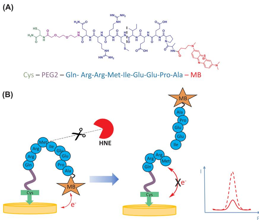
**Fig. 1.** (A) Structure of the methylene blue-tagged peptide probe for HNE. (B) Principle of detection for the peptide-based electrochemical biosensor. HNE catalyzes the cleavage of the methylene blue-labelled peptide substrate releasing the redox containing fragment into solution, leading to a decrease in the electrochemical signal as measured by SWV.
