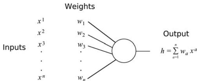
**Figure 1. Setup and definitions.** Binary input vectors  $x^a$  are presented, with each component having probability  $p$  of being in the high state. Synaptic weights  $w_a$  occupy one of  $W$  discrete states, whose values are equidistantly spaced around zero. The output  $h$  is the inner product of the vector of inputs with the weight vector.
