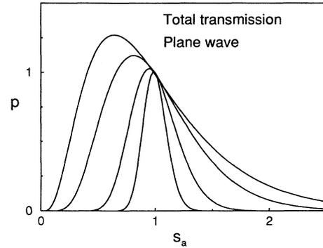
FIG. 2. Intensity distribution of the total transmission, in units of  $\sqrt{3g/2\pi}$ , versus the normalized intensity  $s_a$  for an incoming wave with Gaussian profile.  $g = 2, 4, 16,$  and  $64$  (upper to lower curves).
