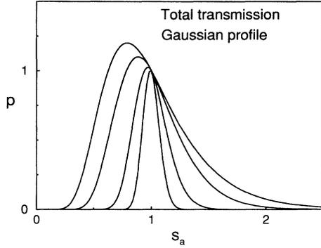
FIG. 1. Intensity distribution of the total transmission, in units of  $\sqrt{3g/4\pi}$ , versus the normalized intensity  $s_a$  for an incoming plane wave.  $g = 2, 4, 16,$  and  $64$  (upper to lower curves).
