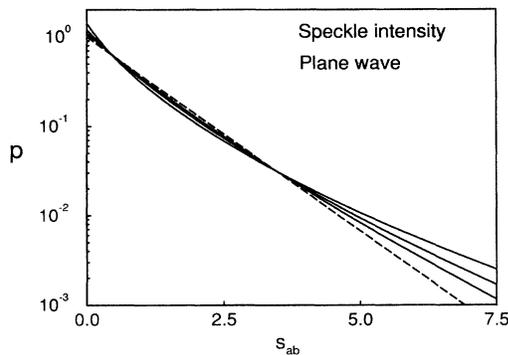
FIG. 3. Intensity distribution of speckles versus the normalized intensity  $s_{ab}$  for an incoming plane wave.  $g = 2, 4,$  and  $8$  (upper to lower curves at  $s_{ab} = 5$ ). The dashed line corresponds to the Rayleigh law ( $g = \infty$ ).
