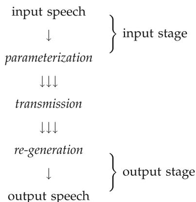
**Figure 1.** A vocoder. The multiple arrows indicate that the parameterized representation of speech typically has several distinct groups of parameters – e.g., filter coefficients capturing the spectral envelope and source parameters such as the fundamental frequency F0.
