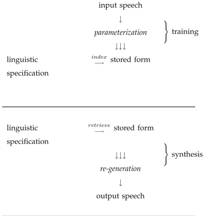
**Figure 2.** Speech synthesis, viewed as a vocoder. The input stage of the vocoder has become ‘training’ and is performed just once for the entire speech corpus (training data). The output stage of the vocoder has become ‘synthesis’, which is performed once for each novel sentence to be synthesized.
