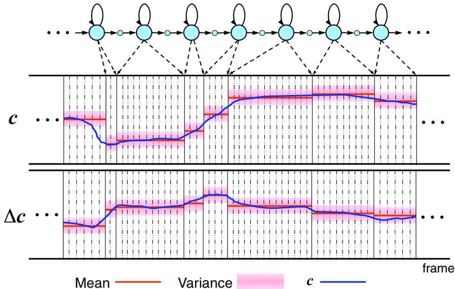
**Figure 3.** Maximum likelihood parameter generation: a smooth trajectory for parameter  $c$  is generated from a discrete sequence of distributions over  $c$ , by taking the distribution over the delta (and delta–delta) coefficients of  $c$  into account. From [http://hts.sp.nitech.ac.jp/archives/2.2beta/HTS\\_Slides.zip](http://hts.sp.nitech.ac.jp/archives/2.2beta/HTS_Slides.zip).
