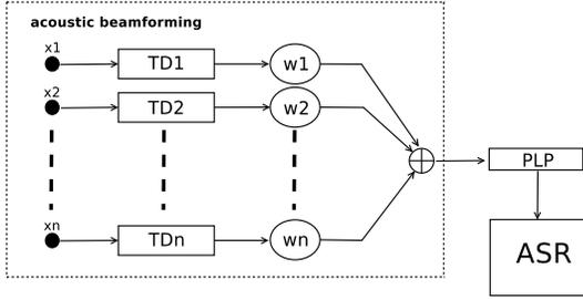
Figure 2: An array-based ASR system using an acoustic delay-sum beamformer.  $x_1, x_2, \dots$  represent microphone elements in the array, and the TD blocks represent time delay compensation for each channel.  $w_1, w_2, \dots$  are weights applied to the channels.
