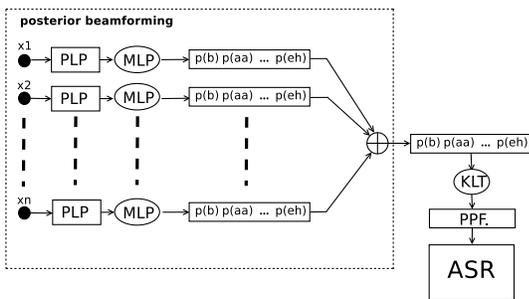
Figure 3: An array-based ASR system using the posterior accumulation approach.  $x_1, x_2, \dots$  represent microphone elements in the array, and  $p(b), p(aa), \dots$  represent the raw posterior probabilities of this frame belonging to phone  $b, aa$ , etc. The posterior probabilities from all channels are accumulated and averaged. A logarithm and KLT transforms them into PPFs.
