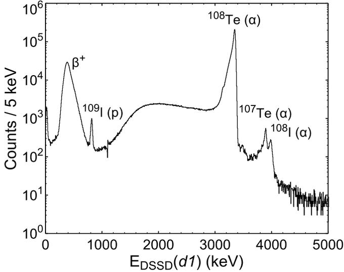
Figure 2: Energy spectrum for all decay events observed as a member of a  $R$ - $d1$  event chain. The previously known activities are labeled. The discontinuity at the energy of 1100 keV is due to the different energy calibration for proton- and  $\alpha$ -decay events.
