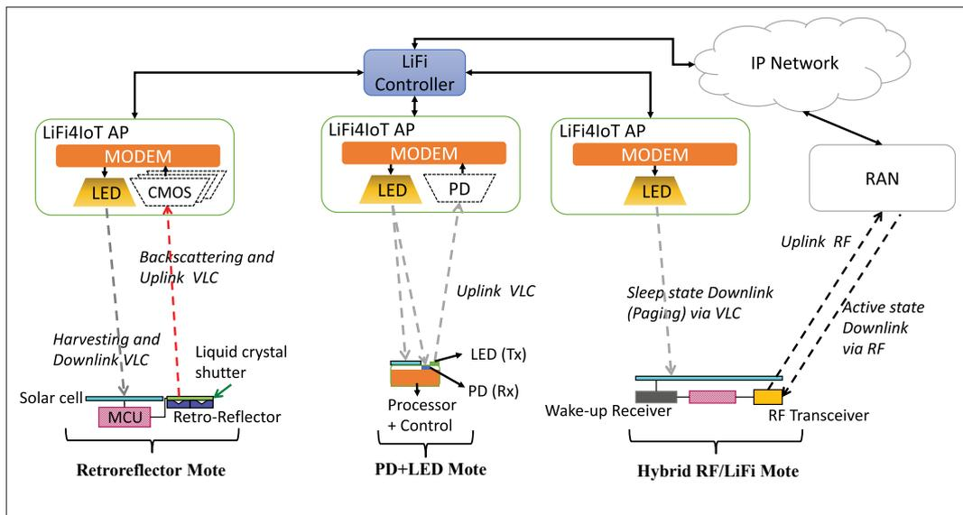
Figure 2. Schematic LiFi4IoT System: LiFi4IoT AP and motes.
