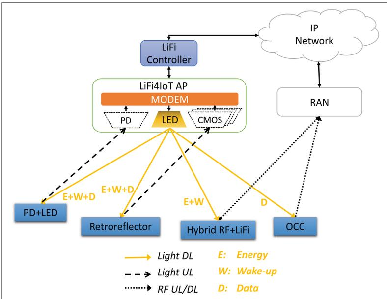
Figure 1. LiFi4IoT system architecture and its working principle.
